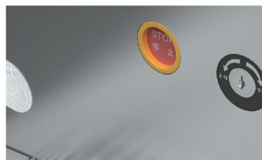
急停按钮 Emergency Stop Button
